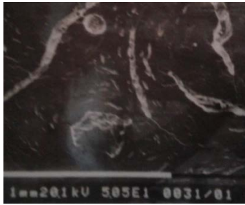
Fig. 1c. Oil coke macrostructure
