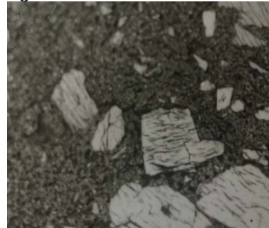
Fig. 1e. Macrostructure of carbonic composite K-1
