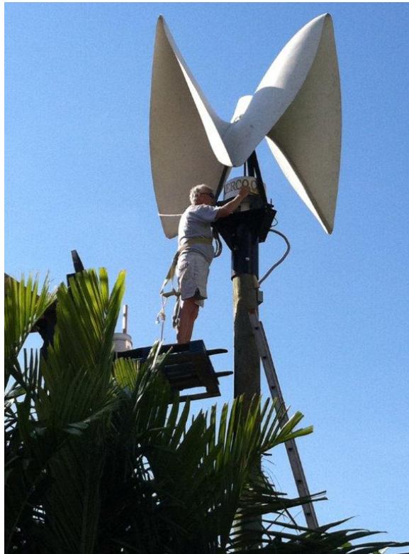
Figure 1: Analyzed wind turbine with vertical axis helical type
